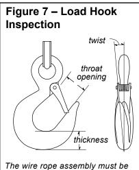
replaced if the throat opening is 15% wider than nominal, if the thickness is 10% less than nominal, or if the hook is twisted 10° or more.
