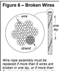
3 wires are broken in one strand in one lay.
